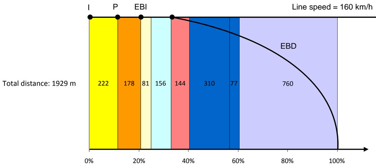
Figure 13: Distance apportionment for Conventional passenger train- gamma approach
