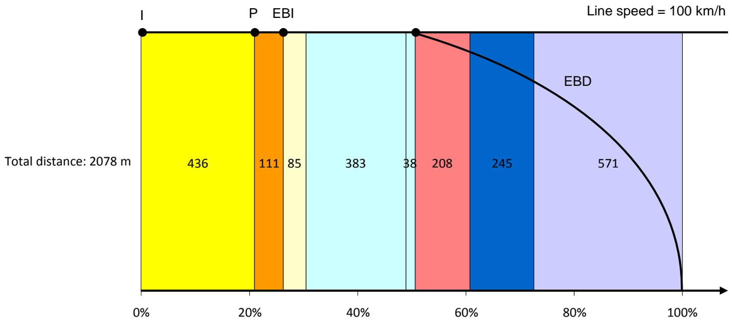
*Figure 16: Distance apportionment for freight train braked in G mode*
