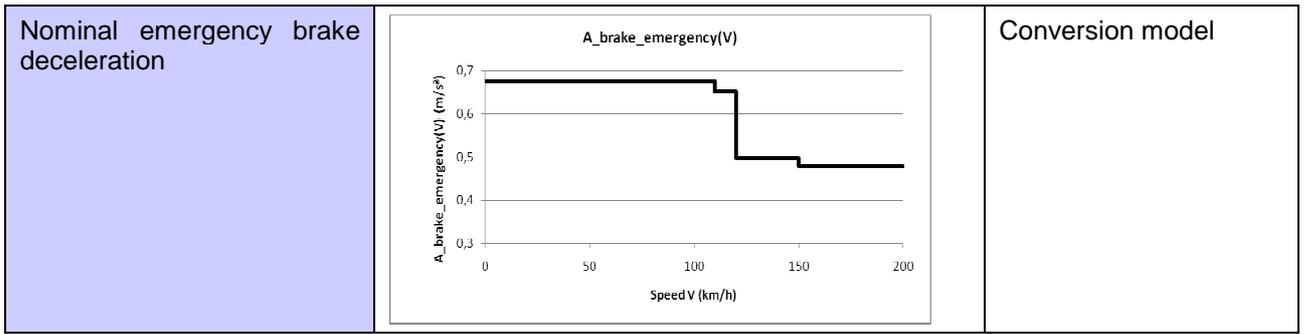
*Table 6: Freight train braked in G mode, example of input parameters*
