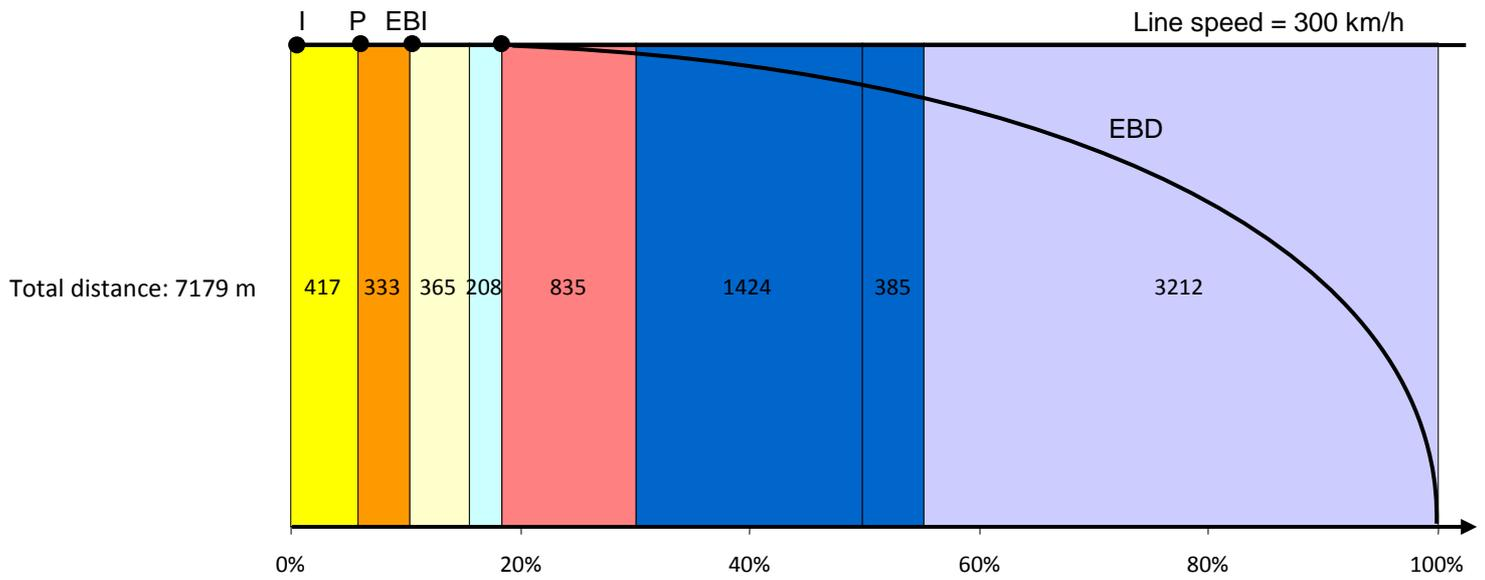
*Figure 12: Distance apportionment for high speed train*
