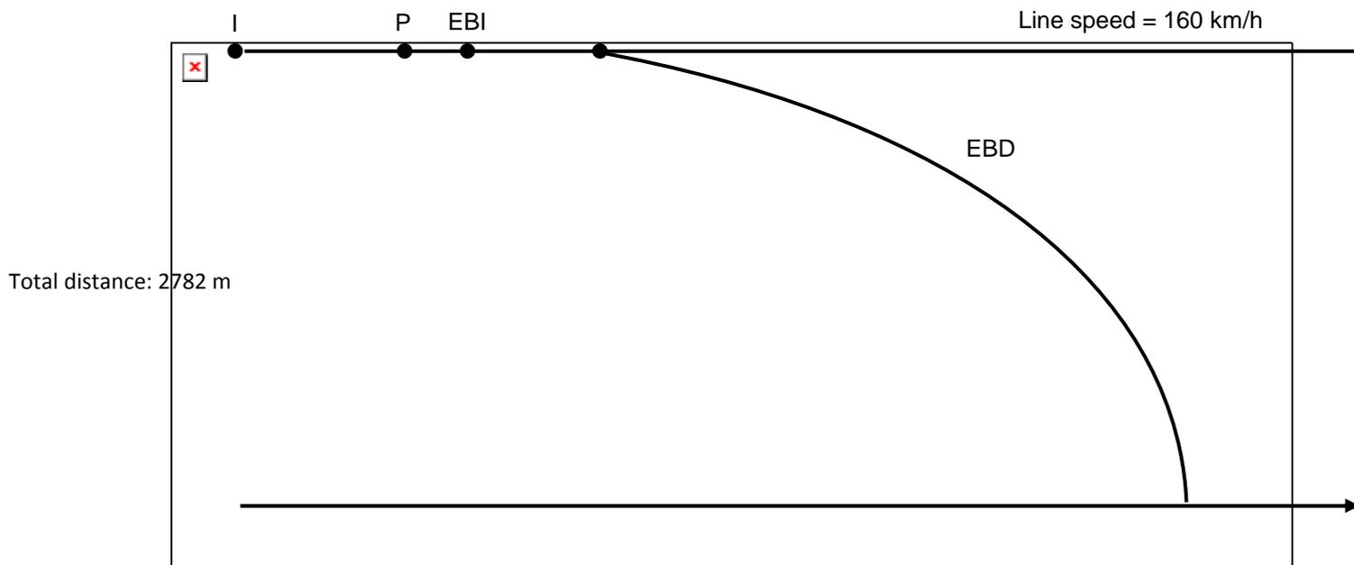
*Figure 15: Distance apportionment for freight train braked in P mode*
