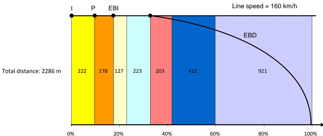
Figure 14: Distance apportionment for Conventional passenger train - lambda approach
