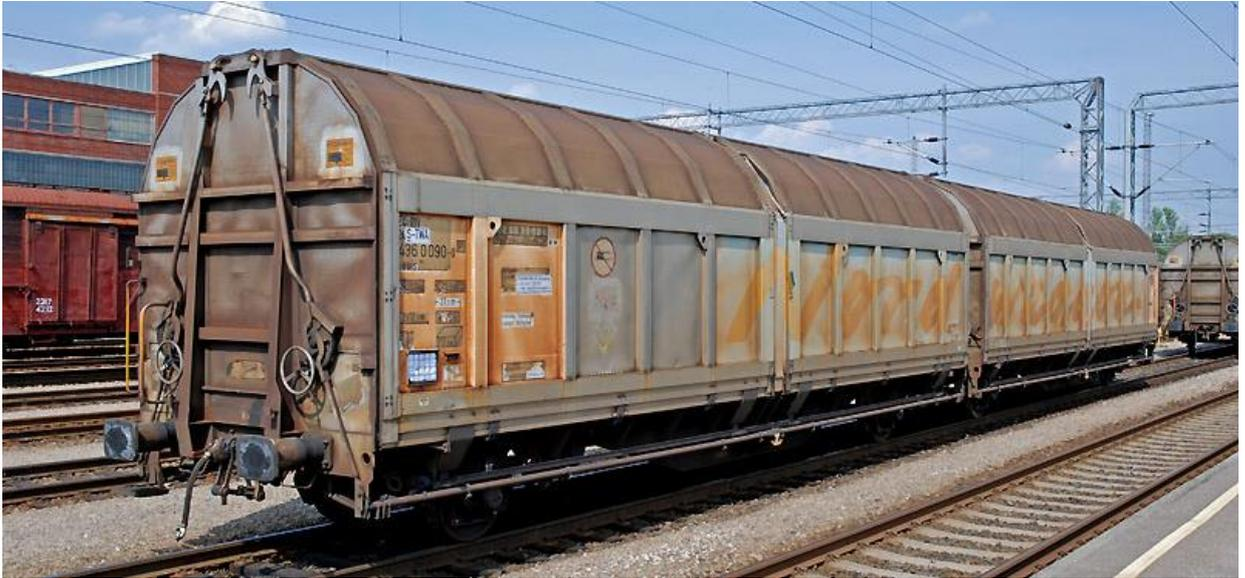
**Figure 4: Example 3 of a unit consisting of a rake of permanently connected elements, those elements cannot be operated separately (self-discharging train)**
