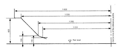
Note: On inclined connections with a radius  $R \geq 500$  m, the vertical measurements shown in diagrams A and B above must be reduced by  $\frac{50\ 000}{R}$  mm (R in m). If  $625 \geq R \geq 500$  m, the measurement 80 in diagram A is cancelled.
