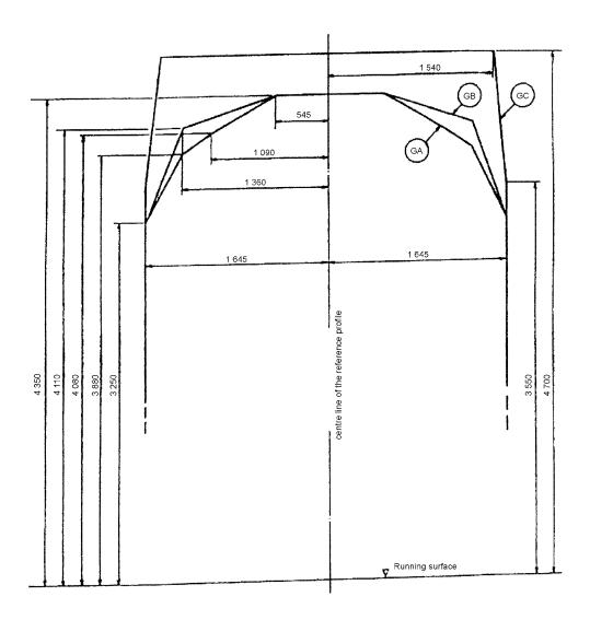
$\textit{N.B.:}\ \text{Up}$  to a height of 3 250 mm, the reference profile of GA, GB and GC gauges is identical.
